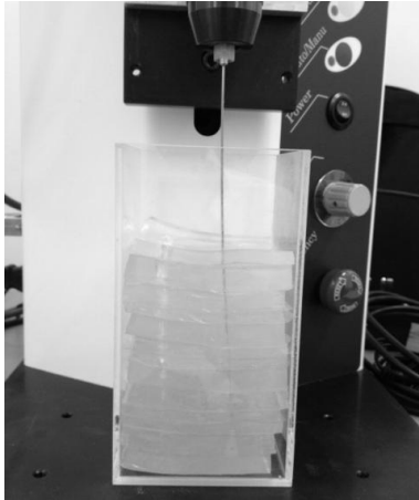
Fig. 7. Multi-layer gelatine sample to simulate the porcine sample.
