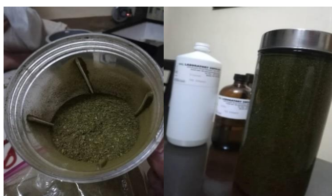
Fig. 2. a). Homogenization of dried C. fistula leaves; b). Maceration in 70% Ethanol
