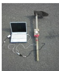
Fig. 8. Hoe connected to sensors and laptop PC.
