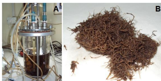
Fig. 2. Cultivation of hairy root culture in a 3-liter Stirred tank reactor. (A) Bioreactor set-up; (B) Hairy roots obtained after 25 d of growth.
