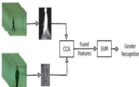
Fig. 4. Face-gait fusion for gender (secondary identifier) extraction
