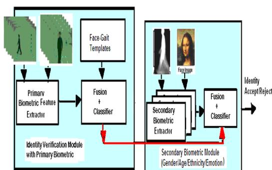
Fig. 6. Fusion structure for primary and secondary identifiers using face and gait patterns.
