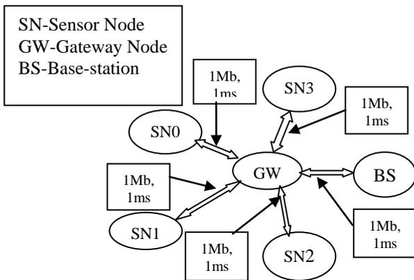
Fig. 1. Transmission loss monitoring of sensor network.
