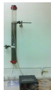
Fig. 4. Set-up for sand-pack column.
