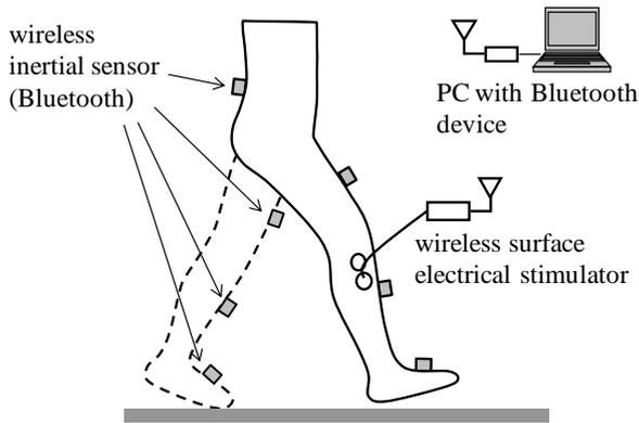
Fig. 1. Outline of an integrated wireless system of FES control and movement measurement.
