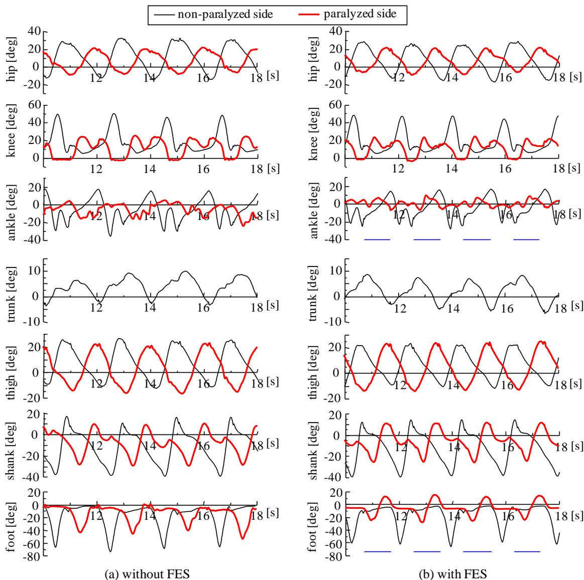
Fig. 3. Examples of measured joint and inclination angles during walking with and without FES assisted foot drop correction (maximum condition). For the FES assisted walking, durations that electrical stimulation was applied are shown by solid lines under the plot.
