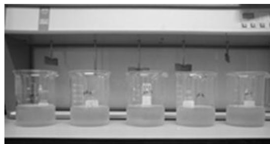
Fig. 3. Jar test with 300 mL of decanted fish canning wastewater for coagulation/flocculation tests.
